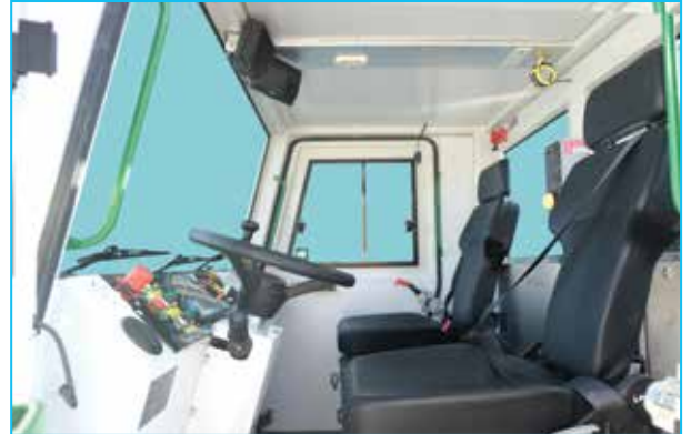
ROPS & FOPS level 2 certified closed 2-person cabin
