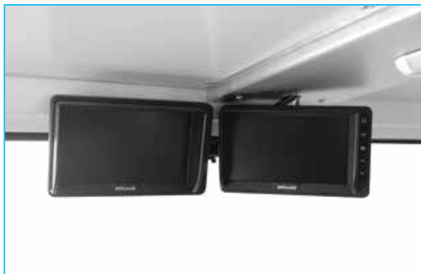
Rear view camera and LCD screen in operator cabin
