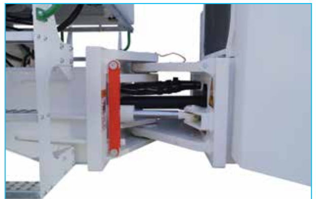
High strength articulated chassis
