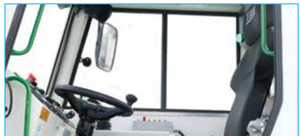
ROPS & FOPS level 2 certified closed 1-person cabin
