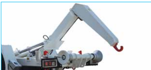
Electronic tracking of hooklift position and angle
