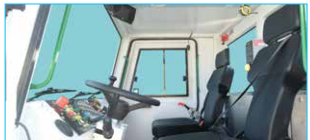
ROPS & FOPS level 2 certified closed 2-person cabin
