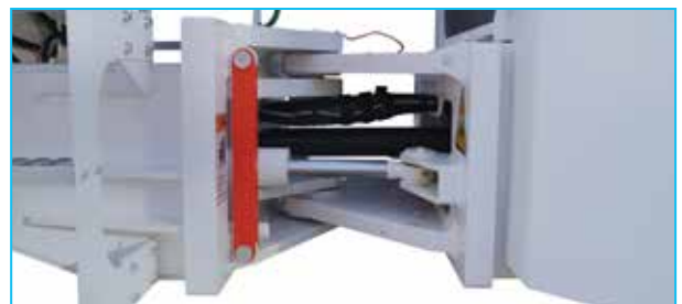
High strength articulated chassis
