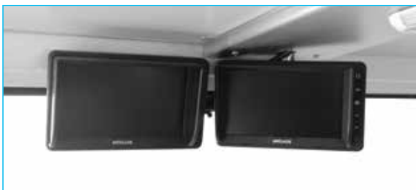
Rear view camera and LCD screen in operator cabin
