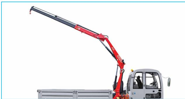
820 kg lifting capacity at 7.1 m
