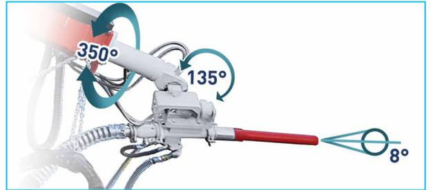
Spraying head with 350° rotation, +/-135° tilt and 8° oscillation
