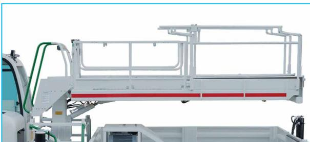
4.5 m +/- 9° height adjustable +/- 95° pivotable telescopic platform
