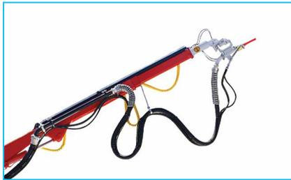
Robust manipulator with 13.5 m vertical and 10.8 m horizontal spraying reach
