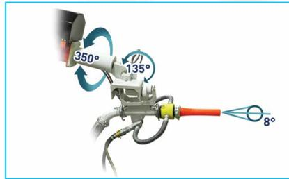
350° rotation +/- 135° tilt and 8° oscillation spraying head
