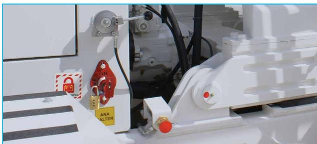
Locked type battery isolator switch
