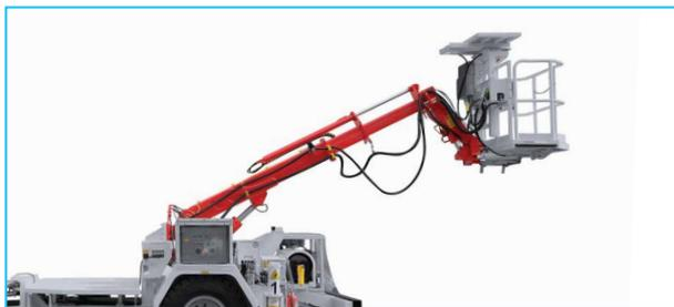
1590 x 790 mm, 500 kg lifting capacity basket
