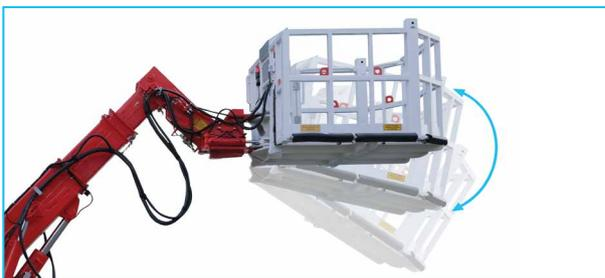
Basket with automatic parallelism conforms to EN280 standard
