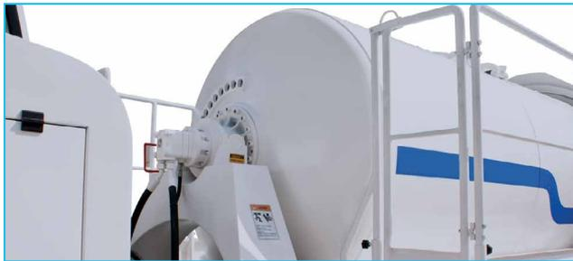
Horizontal drum with 5 m<sup>3</sup> concrete yield
